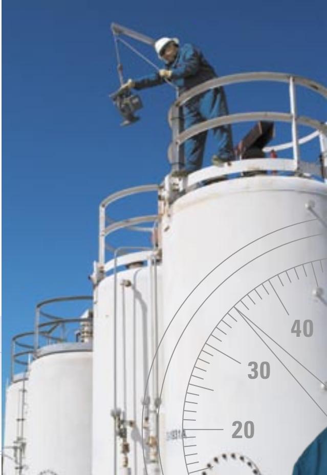
AN ENGINEER IN THE AIR DISTRICT'S SOURCE TEST SECTION, MARCO INSTALLS MONITORING EQUIPMENT AT A GASOLINE DISTRIBUTION TERMINAL. DIRECT MONITORING OF INDUSTRIAL EMISSIONS IS CRITICAL TO THE ENFORCEMENT OF DISTRICT REGULATIONS AND THE PREPARATION OF NEW AIR QUALITY RULES.
